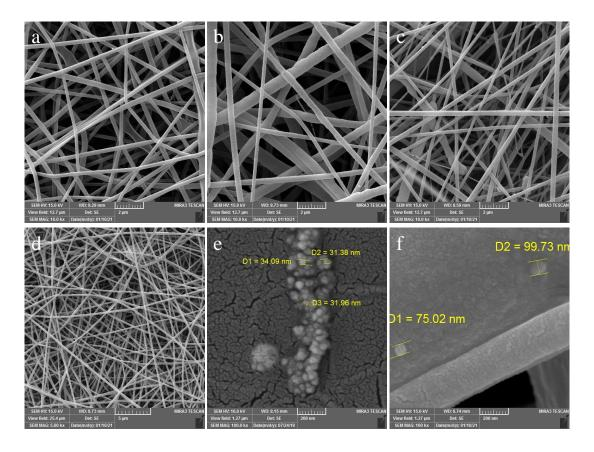
Fig 7. SEM micrographs of the surfaces of (a) Poly vinyl alcohol (PVA) nanofiber, (b) Polycaprolactone (PCL) nanofiber, (c) PVA-PCL nanofiber, (d) PVA-PCL nanofiber containing nanocellulose (NC), (e) bacteriophages, (f) and bacteriophages containing PVA-PCL-NC nanofiber.
