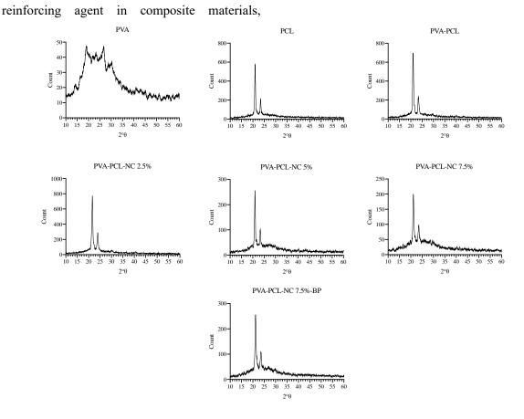
**Fig 5.** X-ray diffraction (XRD) analysis of Polyvinyl alcohol nanofibers (PVA), Polycaprolactone nanofibers (PCL), Polyvinyl alcohol + Polycaprolactone nanofibers (PVA-PCL), and Polyvinyl alcohol + Polycaprolactone + nanocellulose nanofibers at different percentages (PVA-PCL-NC).
