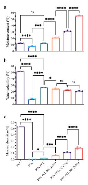
Fig 1. a. Moisture Content, b. Water Solubility, and c. Water Absorption of Nanofibers. Poly vinyl alcohol nanofibers (PVA), Polycaprolactone nanofibers (PVA-PCL), and Poly vinyl alcohol + Polycaprolactone + nanocellulose nanofibers (PVA-PCL-NC). The data, mean  $\pm$  SD (n = 3). NS: not significant, \*\*p < 0.01, \*\*\*\*p < 0.0001, versus multiple comparisons.
