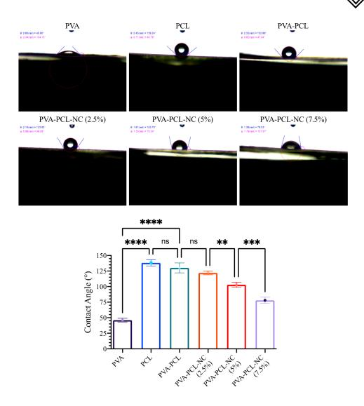
Fig 2. Contact angle measurements of PVA, PCL, PVA-PCL, and PVA-PCL-NC composites with varying concentrations of nanocellulose (2.5%, 5%, and 7.5%). Data are presented as mean  $\pm$  SD (n = 3). Statistical significance: ns: not significant, \*\*p < 0.01, \*\*p < 0.0001.
