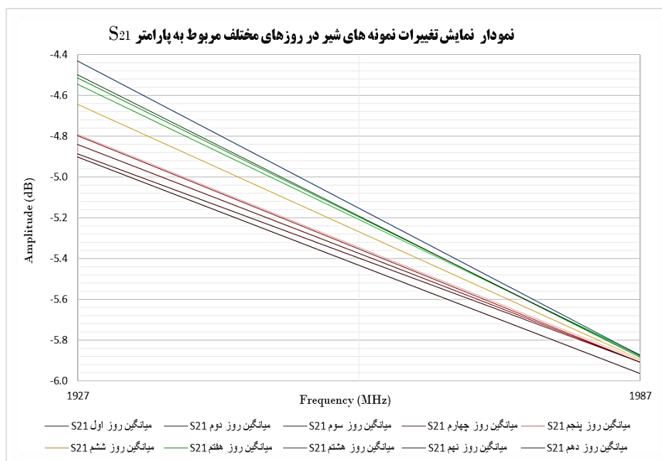
Fig 7. Variations of S21 at frequencies 1867 MHz and 1927 MHz
