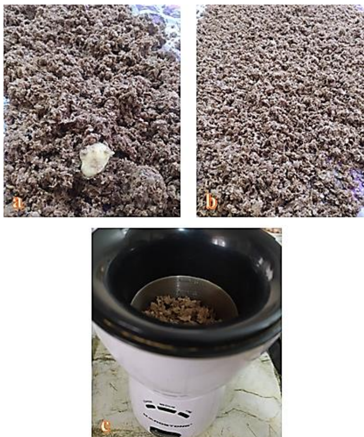
Fig 1. potato peel Preparation process: a) Fresh potato peel samples before washing; b) Dried potato peel samples; c) Grinding dried potato peel samples using a laboratory grinder
