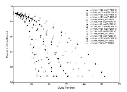
Fig 1. Drying curves of zucchini at different experimental conditions ( $\lambda$ , v and IP are indicative the thickness of samples, air velocity and infrared power, respectively).
