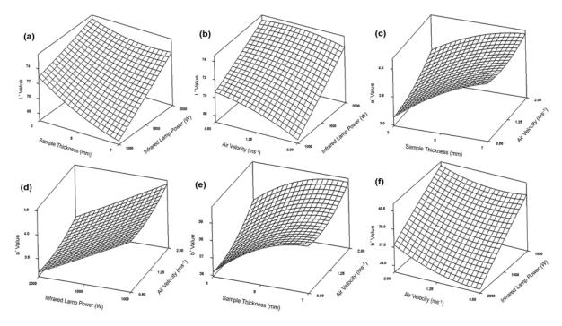
Fig 4. Response surface plots of color parameters at different drying conditions. (a) and (b) L\* values, (c) and (d) a\* values, (e) and (f) b\* values
